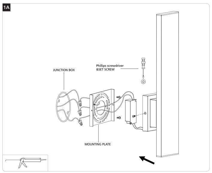
Remove the set screws both sides of the fixture base.
